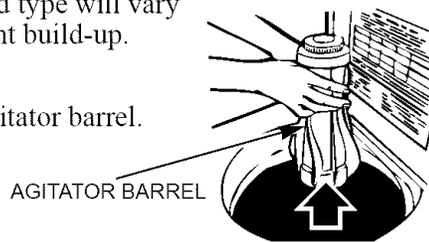
2. Wash or wipe the filter clean in the bottom of the agitator barrel. The filter is not removable.
