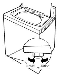
If the washer is not level, adjust the front leveling legs. Turn clockwise to raise, counterclockwise to lower.
