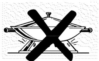
Do not use a wok support ring. Placing the ring over the burner or grate may cause the burner to work improperly, resulting in carbon monoxide levels above allowable standards. This could be dangerous to your health.
