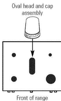
Make sure the slot in the burner head is positioned over the electrode.
