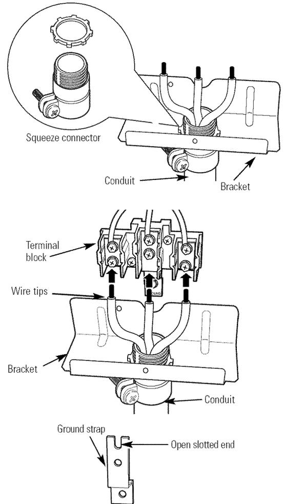
**Wire used, location and enclosure of splices, etc., must conform to good wiring practices and local codes.**
