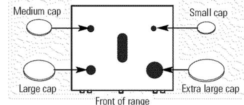
Make sure that the heads and caps are replaced in the correct locations.
