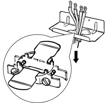
**NOTE:** The replacement power cord must be a 3-conductor or a 4-conductor UL-listed range cord or conduit. Cords may be provided with ring terminals on wire and a strain relief device.
