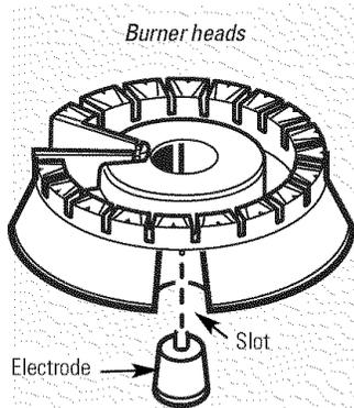
The burner heads are removable. Simply lift them off the range for cleaning.
