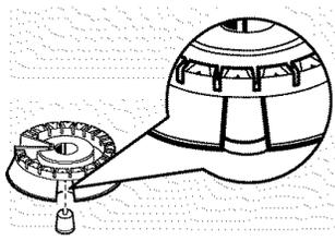
Make sure the slot in the burner head is positioned over electrode.
