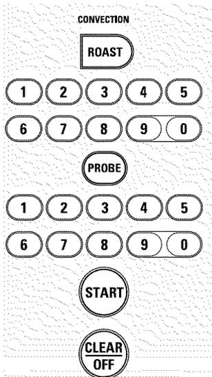
To change the oven temperature during the Convection Roast cycle, touch the **CONVECTION ROAST** pad and then touch the number pads to set the new desired temperature.
