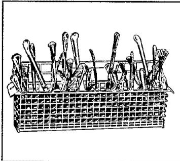
Load knives and fork with handles up. Be sure items do not protrude through the holes in the basket and stop the rotation of the spray arm.
