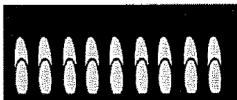
(C) Soft blue flames— Normal for natural gas
