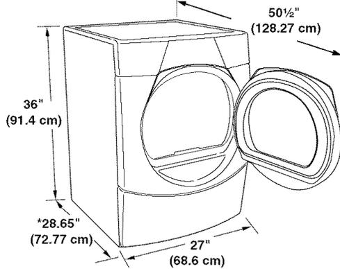
\*Most installations require a minimum 5" (12.7 cm) clearance behind the dryer for the exhaust vent with elbow. See "Venting Requirements."
