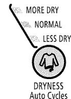
Auto Dry cycles take the guesswork out of drying time and enhances fabric care. The amount of time that is displayed is the estimated time remaining in the cycle.
