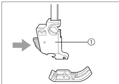
3. Push the black button on the presser foot holder and remove the presser foot.
