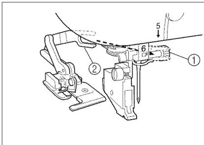
4. Set the fork of the operating lever around the needle clamp screw.
