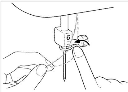
6. Pass the thread through the groove according to the threading sequence (numbers) indicated on the machine.
