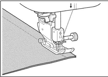
4. When sewing is completed, hold the "Reverse/Reinforcement Stitch" button to sew 3-4 reverse stitches (or reinforcement stitches) at the end of seam.
