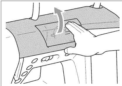
Open the top cover to wind the bobbin or do the upper threading. To open the cover, place your hand under the clear section of the cover and lift up.
