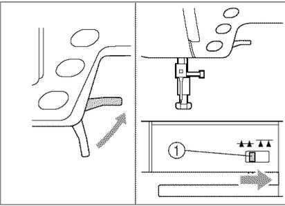
2. Raise the presser foot lever and detach the flat bed table attachment. Move the feed dog position switch to the right to lower the feed dogs.
