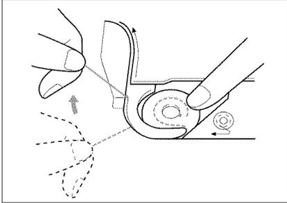
1. Guide the bobbin thread through the groove, following the arrow in the illustration. Do not cut the thread.
