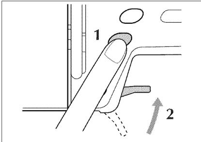
1. Push the "Needle Position" button to raise the needle, then turn off the power.
