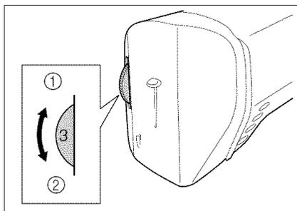
Turn the presser foot dial in order to adjust the pressure applied by the presser foot. The higher the number, the stronger the pressure will be. The presser foot dial has settings from 1 (weakest) to 4 (strongest). Use setting "3" for normal sewing. Lower the presser foot lever before turning the presser foot dial. If you adjust the setting, be sure to return it to "3" after sewing.
