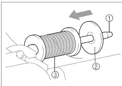
3. Place the spool of thread on the supplemental spool pin, so that thread unrolls from the back. Then push a spool cap onto the spool pin as far as possible to secure the thread spool.
