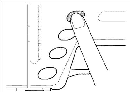
9. Press the “Thread Cutter” button to trim the threads.
