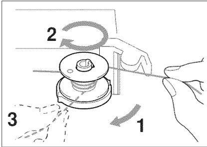
9. Wind the thread clockwise around the bobbin 4-5 times (as shown in the illustration).
