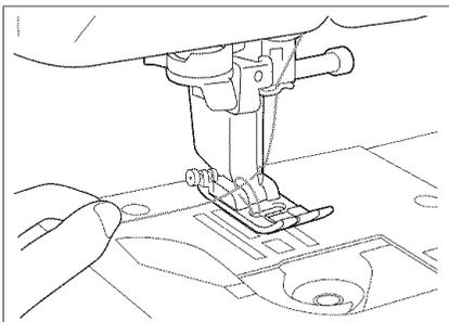
3. Gently pull the upper thread, and a loop of the bobbin thread will come out of the hole in the needle plate.
