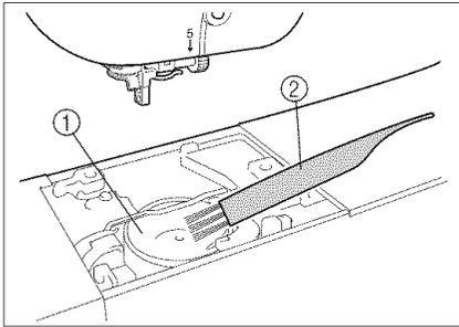
5. Remove accumulated lint and thread from the inner shuttle and race with a brush or vacuum cleaner.
