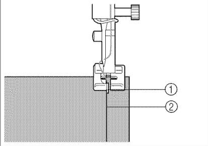
3. Attach blind hem stitch foot "R", and lower the presser foot. Position the fabric so the folded edge touches the guide of the presser foot.
