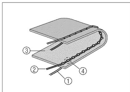
If the upper thread tension is too strong (the bobbin thread can be seen on the top side of the fabric), press the
