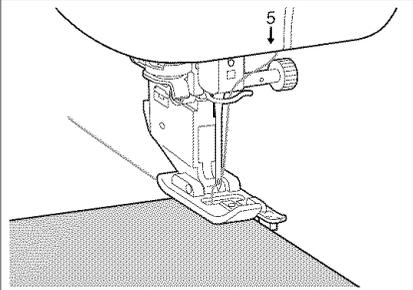
2. Attach presser foot "G". Lower the presser foot so that the presser foot guide is exactly against the edge of the fabric.
