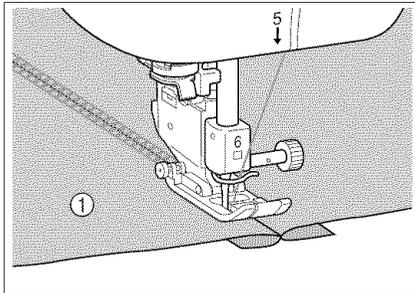
4. Place the fabric right side up in the machine. Center the presser foot over the seam, and sew over the seam.
