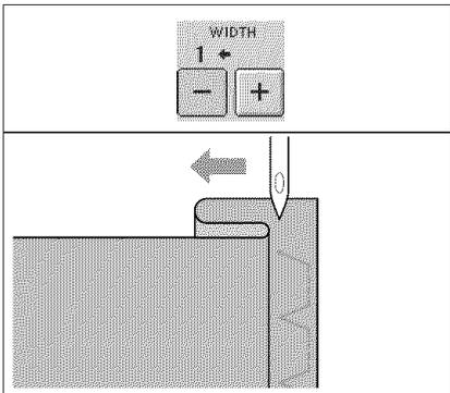
Adjust the width so that the needle slightly catches the fold by pressing **-** in the WIDTH display.
