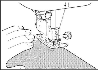
2. Attach presser foot "J". Hold the thread tails and fabric with your left hand, and turn the balance wheel with your right hand to insert the needle into the fabric. This is the sewing start position.
