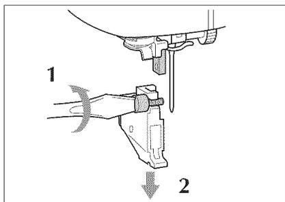
4. Use the included screwdriver to loosen the screw of the presser foot holder, then remove the presser foot holder.
