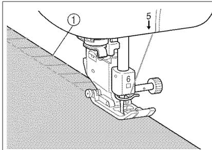
2. Attach presser foot "J". Sew with the needle dropping slightly off the edge of the fabric.
