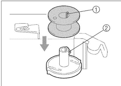
1. Align the groove in the bobbin with the spring on the bobbin winder shaft, and set the bobbin on the shaft.
