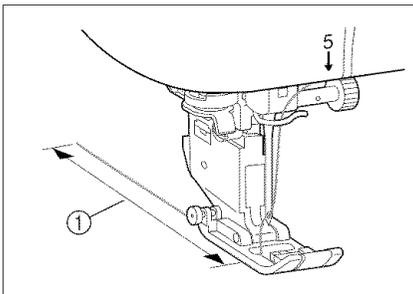
15. Pass the thread under the presser foot, and pull it about 100 mm (3 inch - 4 inch) toward the back of the machine.
