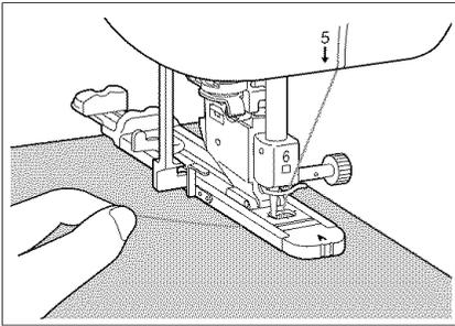
5. Gently hold the end of the upper thread, and then press the "Start/Stop" button to start the machine. Once sewing is completed, the machine automatically sews reinforcement stitches, and then stops.
