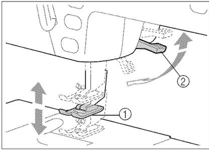
Lower the presser foot lever to lower the presser foot and apply pressure to the fabric. If the presser foot is raised to the second position, and you want to sew heavy weight, stacked fabrics, etc., that are hard to set under the presser foot, raise the presser foot lever higher and hold it to make room for the fabric (see page 2-4).
