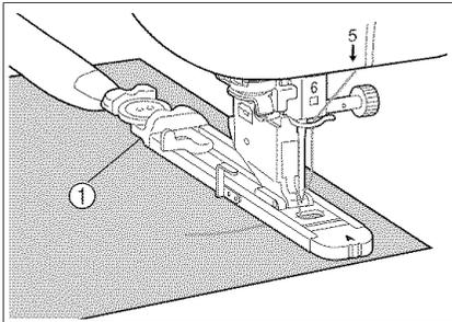
3. Attach buttonhole foot "A". Pull out the button holder plate on the presser foot, and insert the button that will be put through the buttonhole, then tighten the button holder plate around the button.
