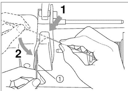
5. Hold the thread from the spool in both hands, and pass the thread around the plate in the thread guides. Use both hands to set the thread around the thread guide plate.
