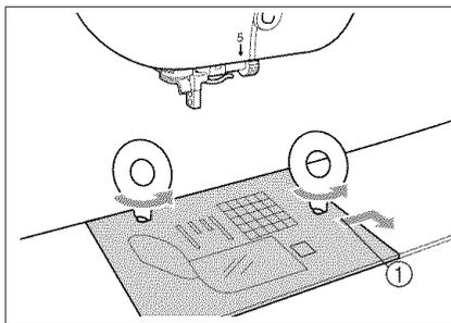
2. Loosen the screws with the disc-shaped screwdriver and remove the needle plate.
