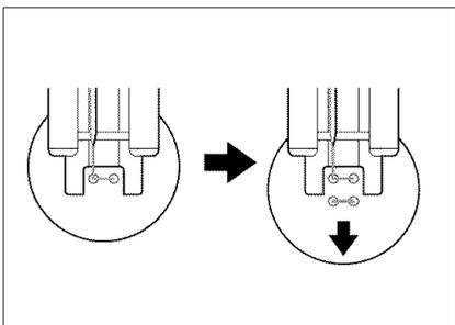
Sew the two holes closest to you. Then raise the presser foot lever and move the fabric so that the needle goes into the next two holes, and sew them in the same way.
