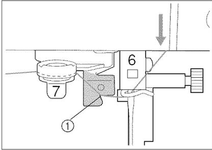
9. Set the thread securely into the slit of the disk in the thread guide. Be sure that the thread catches the corner of the thread guide.
