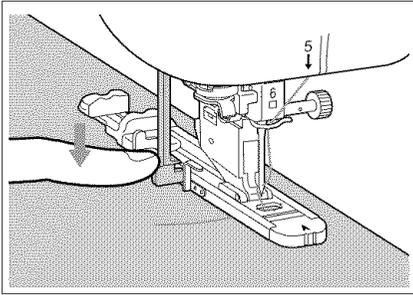
4. Lower the buttonhole lever so that it is positioned behind the metal bracket on the buttonhole foot.
