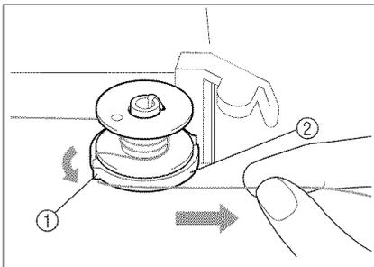
10. Pass the end of the thread through the guide slit in the bobbin winder seat, and pull the thread to the right. The cutter will cut the thread.
