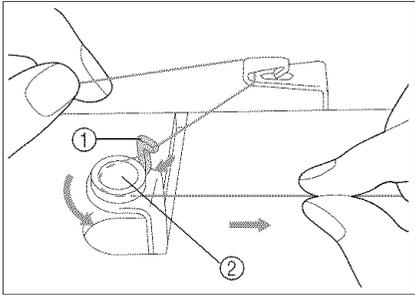
5. Pass the thread around the projection in the thread guides, then pass the thread under the pretension disk. Make sure to set the thread securely under the pretension disk.
