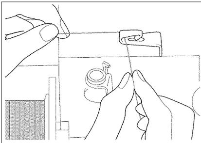
6. Hold the thread from the spool with both hands, and set the thread in the thread guide.
