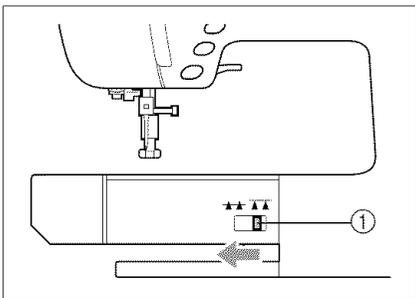
6. When sewing is completed, be sure to return the feed dog position switch to its original position.
