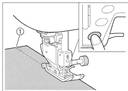
3. Set the fabric in the start position and start sewing. The machine will automatically sew reverse stitches (or reinforcement stitches) and then continue sewing.
