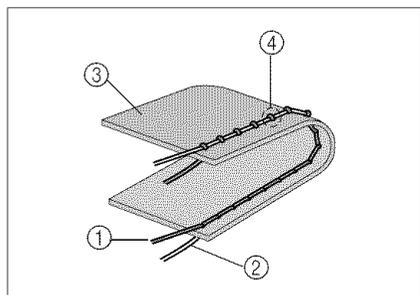
If the upper thread tension is too weak (the upper thread can be seen on the bottom side of the fabric), press the
