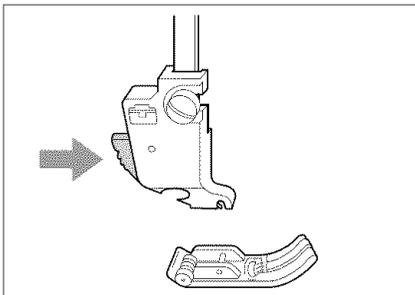
3. Press the black button on the presser foot holder, and remove the presser foot.
