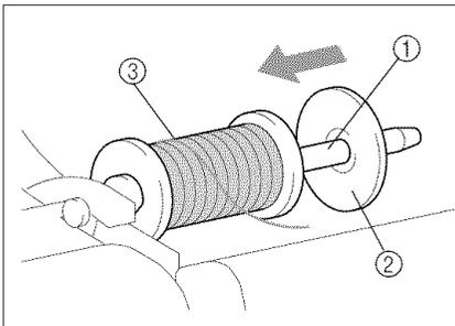
5. Place additional spool of thread on the supplemental spool pin, so that the thread unrolls from the back. Then insert a spool cap onto the spool pin all the way in, to secure the thread spool.
