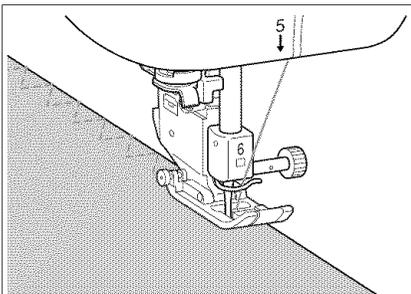
Use this stitch to sew overcasting on the edge of stretch fabrics. Sew the overcasting along the edge of the fabric with the needle dropping off the edge of the fabric at the right.
