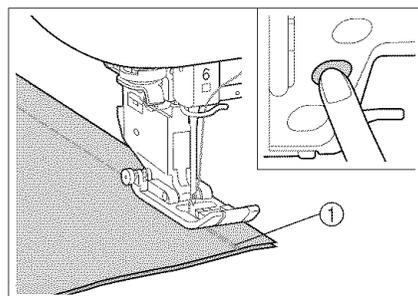
4. Press the "Reverse/Reinforcement Stitching" button. The machine will sew reverse stitches (or reinforcement stitches), then trim the thread.
