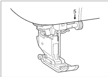
5. With the presser foot lever raised, tighten the screw lightly to attach the presser foot holder.
