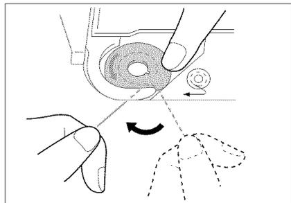
3. Put the bobbin in the shuttle, making sure the thread unrolls as shown.
