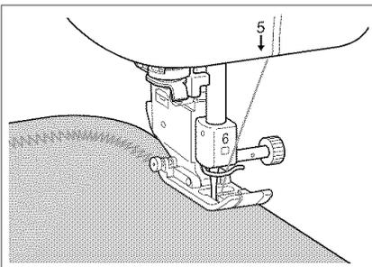
Shorten the stitch length setting to obtain a fine stitch. Sew slowly, keeping the seams parallel with the fabric edge as you guide the fabric around the curve.
