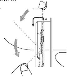
8. Set the thread behind the needle clamp thread guide on the needle bar. To set the thread easily, hold the end of the thread with your left hand, and use your right hand to guide the thread behind the needle clamp thread guide.
