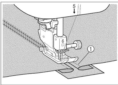
3. Attach presser foot "J". Align the center of the presser foot with the middle of the space between the fabrics and begin sewing. Use a thick thread.
