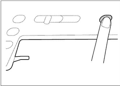
12. Press the "Bobbin Winder" button to start winding the bobbin.
