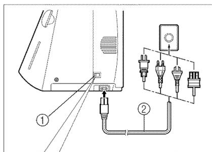
1. Insert the power cord into the cord jack, then insert the plug into a wall outlet.
