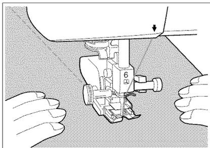
3. Place one hand on each side of the presser foot to hold the fabric securely. Sew while holding the fabric.
