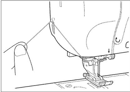
10. Use the thread cutter on the side of the machine to cut the thread.
