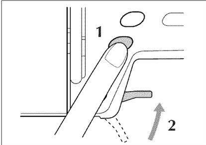
1. Push the "Needle Position" button to raise the needle, then turn the main power switch to OFF.
