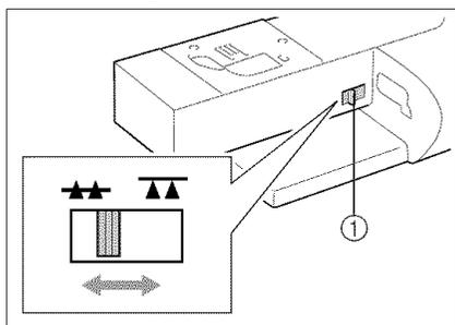
Use this switch when attaching buttons (see page 3-61) or for other similar projects. Remove the flat bed attachment and raise the presser foot lever to operate the feed dog position switch. Set the lever in the **▲▲** position for normal sewing
