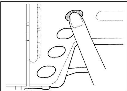
5. After sewing, press the "Thread Cutter" button to trim the threads.
