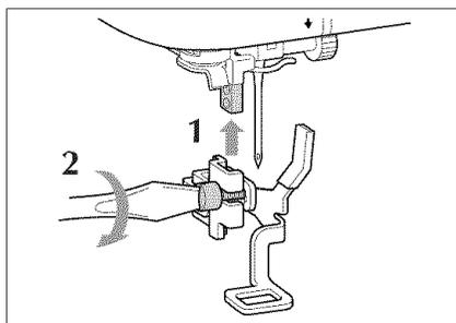
5. Set embroidery foot "Q" on the presser foot bar so that the arm of embroidery foot "Q" is in contact with the back of the needle holder, then use the included screwdriver to firmly tighten the screw.
