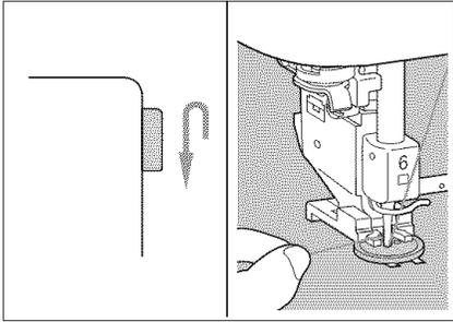
4. Turn the balance wheel to check that the needle goes into each hole correctly. Then, gently hold the end of the upper thread and start sewing. The machine stops automatically when sewing is finished.
