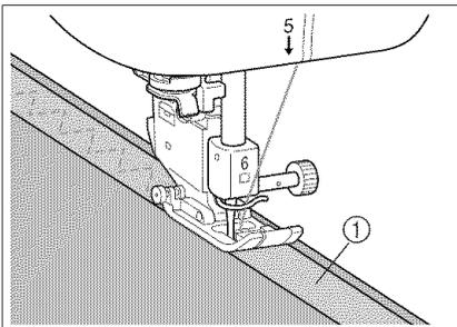
Stretch the tape flat. While stretching the tape flat, sew the tape to the fabric.
