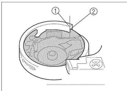
3. Turn the balance wheel, and align the notch of shuttle a little to the left of the shelf of race, as shown.
