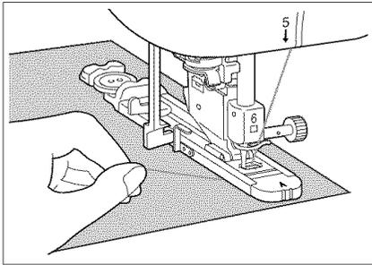
6. Gently hold the end of the upper thread, and then start sewing. Feed the fabric carefully by hand while the buttonhole is sewn. Once sewing is completed, the machine automatically sews reinforcement stitches, and then stops.
