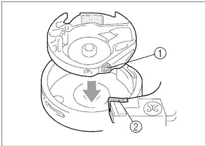
6. Check that the notch on the shuttle is in the same position as when you removed the race. Position the race so that the shelf and spring are aligned, and insert the race.
