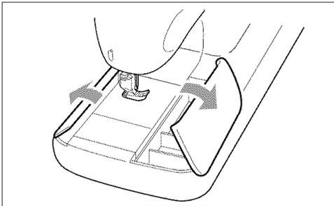
Pull the top of the flat-bed attachment towards you to open the accessory compartment.
