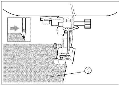
3. Attach presser foot "J". Check that the needle drops slightly off the edge of the appliqué, then begin sewing.
