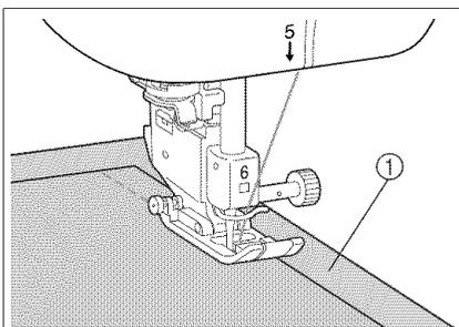
Place thin paper under thin fabrics to make sewing easier. Gently tear off the paper or the stabilizer for embroidery after sewing.
