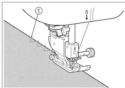
Sew the overcasting along the edge of the fabric so that the right-hand side needle drop point is over the edge of the fabric.
