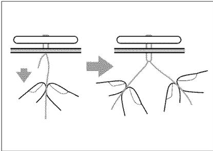
5. From the wrong side of the fabric, pull the end of the bobbin thread to pull the upper thread through to the wrong side of the fabric. Tie the two thread ends together and cut the threads.
