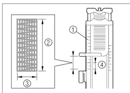
2. Attach buttonhole foot "A" and set the scale to the desired length of the darning.
