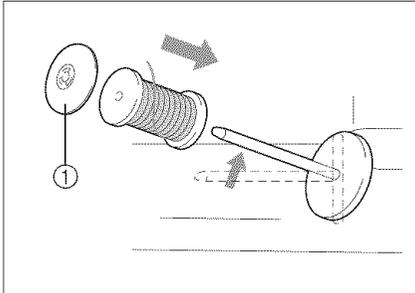
3. Pivot the spool pin so that it angles toward the front of the machine. Set the thread spool on the spool pin so that the thread unrolls from the front of the spool.
