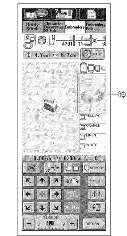
① Bobbin thread sensor: Shows how much thread is left in the bobbin during sewing. The display turns yellow if there is little thread remaining.
