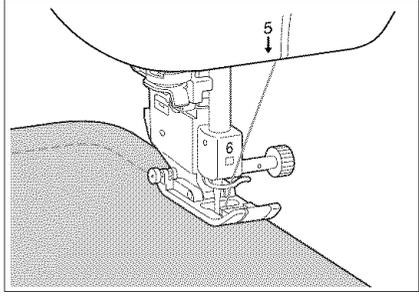
Sew slowly while keeping the seam parallel with the fabric edge as you guide the fabric around the curve.
