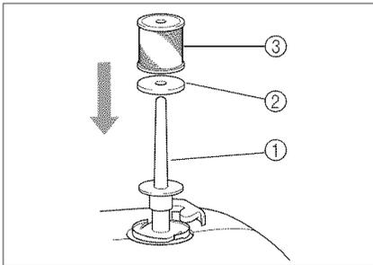
1. Insert the vertical spool pin into the end of the bobbin winder shaft.
