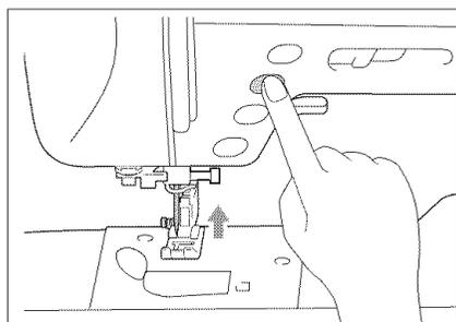
2. Press the "Needle Position" button to set the needle in the up position.
