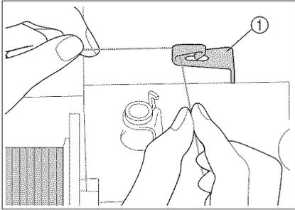
4. With your left hand, hold the thread near the thread spool. With your right hand, hold the end of the thread, and use both hands to set the thread around the thread guides.
