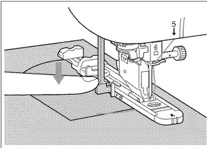
5. Lower the buttonhole lever so that it is positioned behind the metal bracket on the buttonhole foot.
