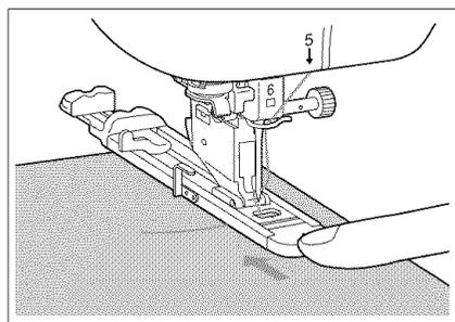
3. Check that the needle drops at the desired position and lower the presser foot lever, making sure the upper thread passes underneath the buttonhole foot.
