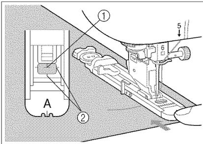
4. Align the presser foot with the mark on the fabric, and lower the presser foot lever.
