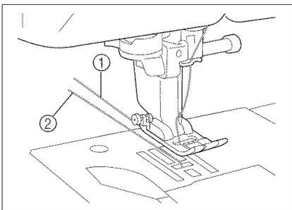
4. Pull up the bobbin thread, then pass it under the presser foot and pull it about 100 mm (3-4 inch) toward the back of the machine, matching the upper thread.
