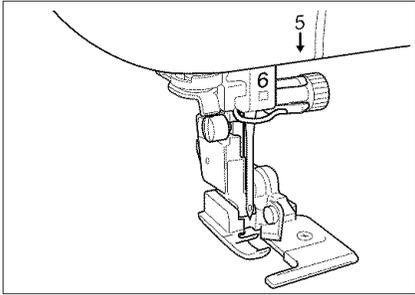
5. Slowly lower the presser foot lever, and then position the pin on the presser foot (side cutter) in the notch of the presser foot holder to attach the presser foot (side cutter).
