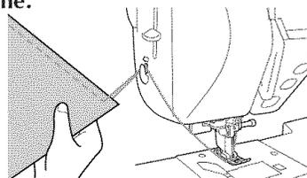
10. When the needle has stopped moving, raise the presser foot and remove the fabric.
