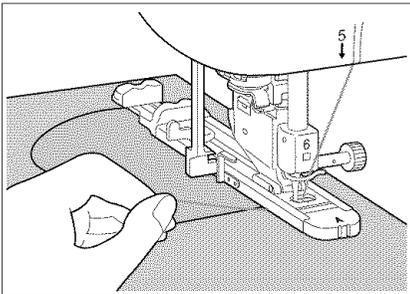
6. Gently hold the end of the upper thread and begin sewing. When sewing is completed, the machine will sew reinforcement stitches and stop automatically.
