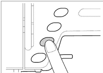
2. Attach presser foot "J". Press the "Reverse/ Reinforcement Stitch" button to sew reinforcement stitches, then continue sewing.
