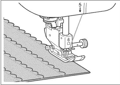
4. Attach presser foot "J". Set the needle drop point slightly off the edge of the fabric, and start sewing.
