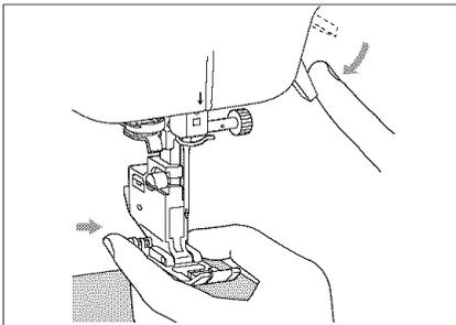
If the fabric does not feed when starting to sew or when sewing thick seams, press the black button on the left side of presser foot "J".
