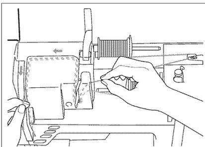
7. Set the thread around the thread guide plate, then pass the thread through the groove according to threading sequence (numbers) indicated on the machine.
