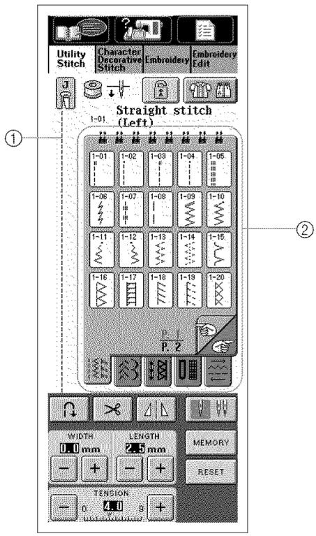
1. Turn the main power switch to ON. The screen shown at left is displayed. The often-used "1-01 Straight (left)" stitch pattern is automatically selected.
