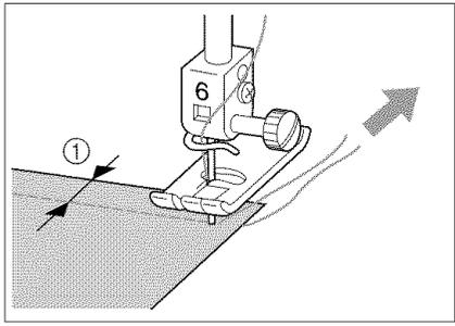
When edge stitching a short stitch length and close to the edge of the fabric, the presser foot may not cover enough fabric for proper feeding. Before you begin to sew, sew a basting thread at the corner point. When you change direction at the corner, start sewing as you pull the basting thread toward the back.
