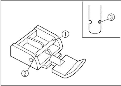
4. Remove presser foot "J". Align the right side of the pin in zipper foot "I" with the presser foot holder, and attach the zipper foot.
