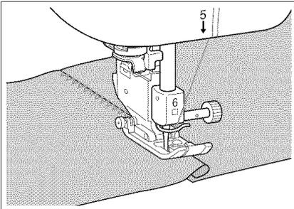
Turn back the desired width of fabric and position it over the lower fabric, then sew so that the stitch bridges both pieces of fabric.
