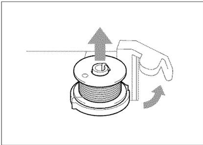
13. The bobbin will stop rotating automatically when it is done winding, and the bobbin holder will return to the original position.
