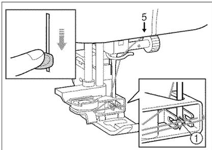
12. Push down the needle threader lever as far as possible. The hook will rotate and pass through the eye of the needle. Make sure that the hook does not catch the fabric or any other objects near the presser foot.
