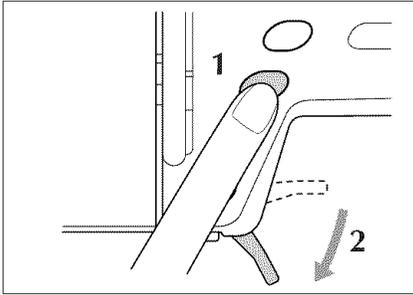
1. Press the "Needle Position" button to raise the needle, then turn the main power switch to OFF.
