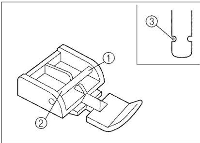
7. Remove the presser foot, and reattach it so that the left side of the pin is attached to the presser foot holder.
