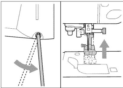
Use your knee to move the knee lifter to the right in order to raise the presser foot. Release to the left for the presser foot to lower.
