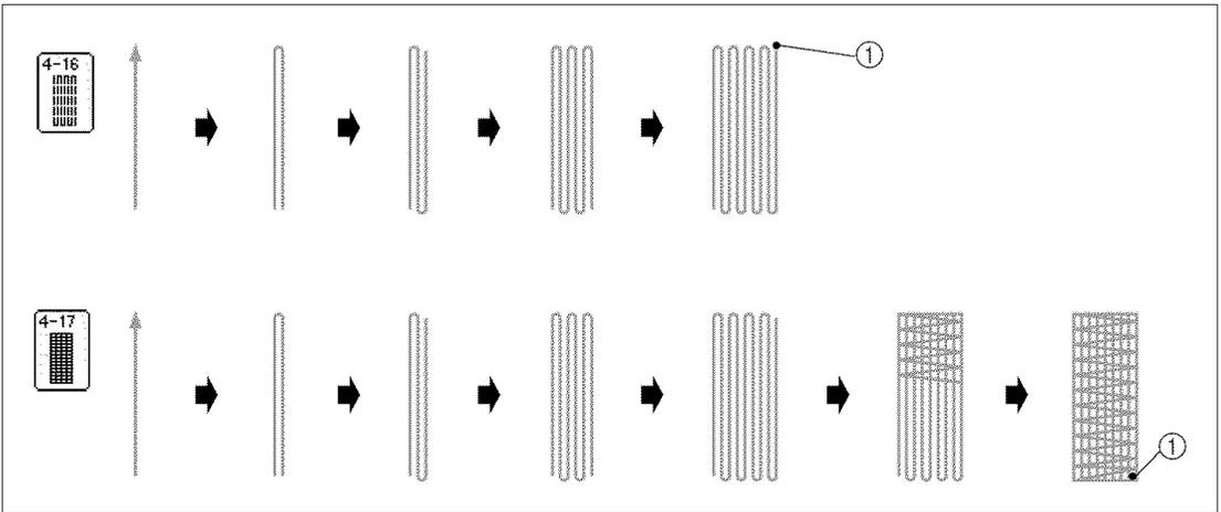
① Cycle of reinforcement stitches
