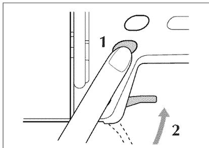
1. Press the "Needle Position" button to set the needle in the up position, and then turn off the main power switch.
