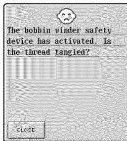
26. This message is displayed when the bobbin is being wound, and the motor locks because the thread is tangled, etc.
