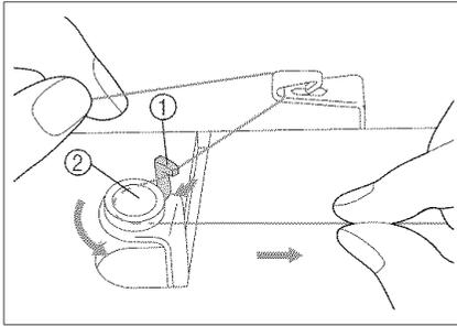
8. Pass the thread around the thread guide shaft and the pretension disk as indicated on drawing. Make sure that thread is correctly inserted inside the pretension disk.
