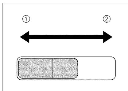
4. Set the speed control slide to control the stitch width.
