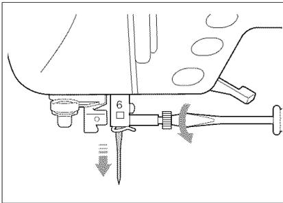
3. Use the screwdriver to turn the screw toward the front of the machine and loosen the screw, then remove the needle.
