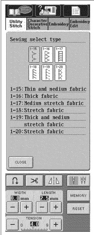
3. The upper part of the screen displays a selection of overcasting stitches with explanations. Read the explanations and select the appropriate stitch.
