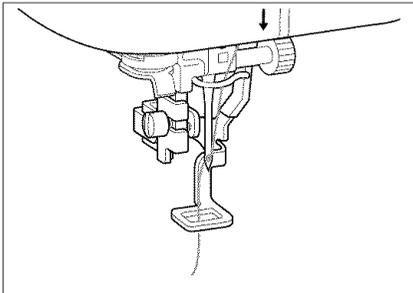
1. Thread the machine with the first color, and pass the end of the thread through the hole in embroidery foot "Q".
