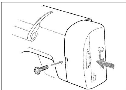
4. Place light cover and tighten the screw on the back of the machine.
