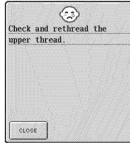
3. This message is displayed when the upper thread is broken or not threaded correctly, and the “Start/Stop” button or the “Reverse/Reinforcement Stitch” button is pressed.
