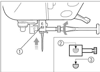
4. With the flat side of the needle facing the back, insert the new needle all the way to the top of the needle stopper (viewing window) in the needle clamp. Use a screwdriver to securely tighten the needle clamp screw.
