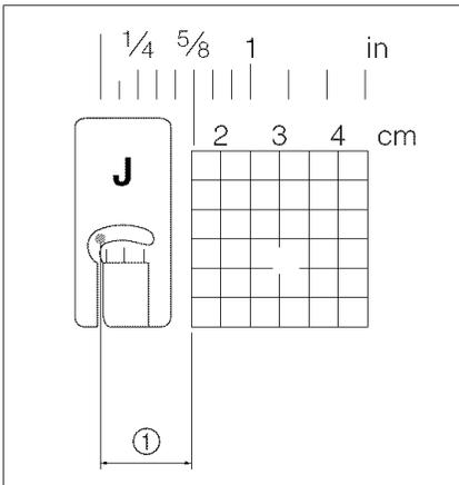
For standard 16 mm (5/8 inch) seam allowance, set **WIDTH 3.5 mm** on LCD.
