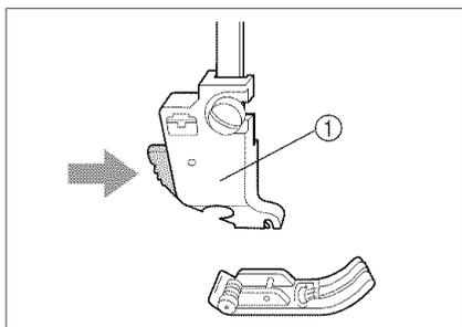
3. Press the black button at the back of the presser foot holder. The presser foot comes off.
