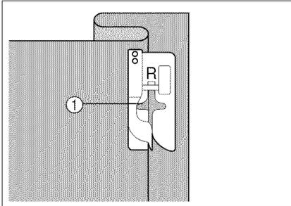
4. Sew the fabric, keeping the folded edge in contact with the presser foot.
