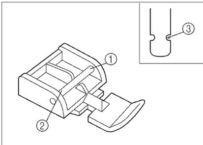
4. Remove presser foot “J”. Align the right side of the pin in zipper foot “I” with the presser foot holder, and attach the presser foot.
