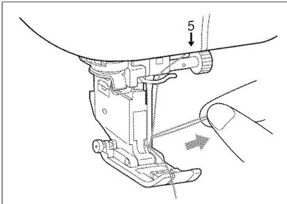
14. Pull the thread loop toward the back of the machine.
