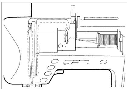
2. Do the upper threading. Follow the steps for threading a single needle for the first threading (see page 1-32 “Upper Threading”).
