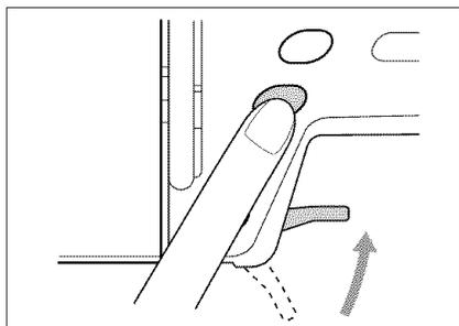
1. Press the "Needle Position" button to raise the needle, and then turn off the power.
