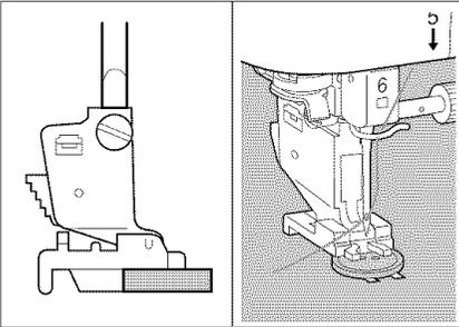
3. Attach button sewing foot "M", place the button in the presser foot, and lower the presser foot lever.
