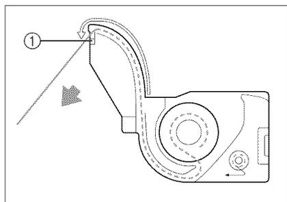
4. Guide the thread through the groove, then pull the thread toward you to cut off any excess.
