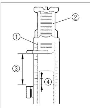
Use the markings on the presser foot scale to set the size of the buttonhole. One mark on the presser foot scale equals 5 mm (3/16 inch).
