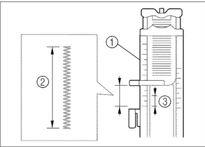
2. Attach buttonhole foot "A" and set the scale to the length of the bar tack you wish to sew.
