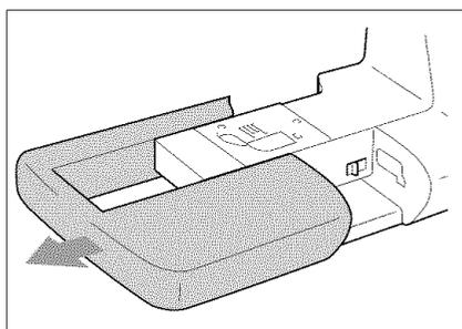
Use the free arm sewing option to attach cuffs, hem pant legs, and sew other tubular pieces. Pull the flat bed attachment to the left to remove it and create the convenient free arm sewing mode.
