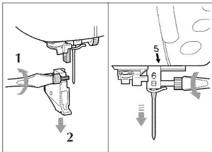
1. Turn off the power. Remove the presser foot holder and the needle.
