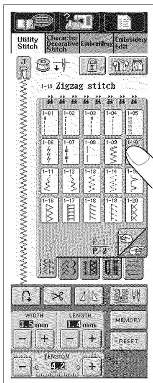
Press a key with your finger to select the stitch pattern, or to select a machine function, or operation indicated on the key.
