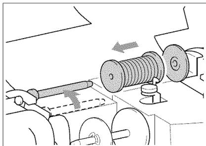
Use this spool pin to wind the bobbin thread during sewing, or when sewing with the twin needle (see pages 1-29, 2-5).
