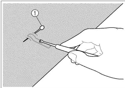
7. Insert a pin along the inside of one of the bar tacks, and then insert the seam ripper into the center of the buttonhole and cut towards the pin.
