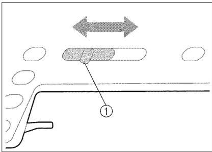
Use this controller to adjust the sewing speed. Move the lever to the left to sew at slower speeds. Move the lever to the right to sew at higher speeds.
