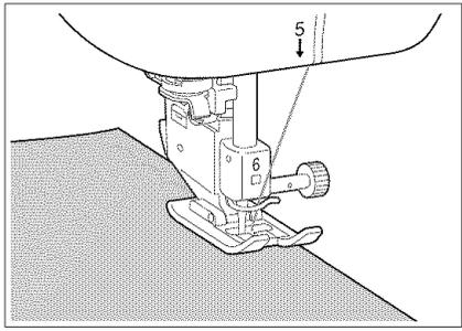
2. Attach presser foot "N". Sew scallop stitches along the edge of the fabric. Do not sew directly on the edge of the fabric.
