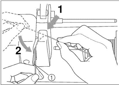
5. Hold the thread from the spool in both hands, and pass the thread behind the thread guide cover on top of the machine.
