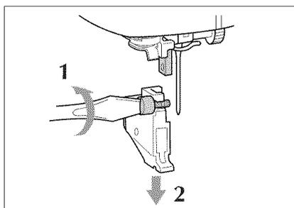
4. Loosen the screw of the presser foot holder to remove the presser foot holder.
