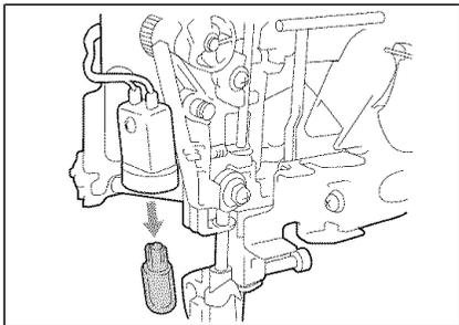
3. Remove the light bulb as shown, and align the projection on the light bulb with the notch in the socket. Replace it with a new light bulb.
