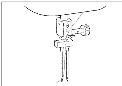
3. Pass the thread through the needle clamp thread guide on the needle bar, then thread the needle on the left side.
