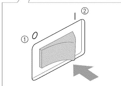
2. Turn the main power switch to "I" to turn on the machine.
