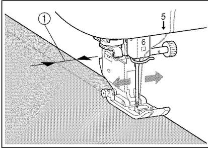
When you select left needle position stitch patterns, you can use **-** and **+** in the Stitch Width display to change the position of the needle. Match the distance from the right edge of the presser foot to the needle with the stitch width, then align the edge of the presser foot with the edge of the fabric during sewing for an attractive finish.
