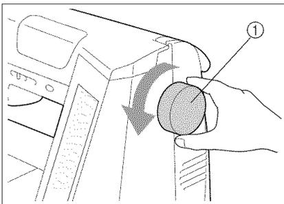
Turn the balance wheel to raise or lower the needle. The wheel should be turned toward the front of the machine.
