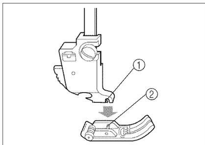
4. Place the new presser foot under the holder, aligning the foot pin with the notch in the holder. Lower the presser foot lever so that the presser foot pin snaps into the notch in the holder.
