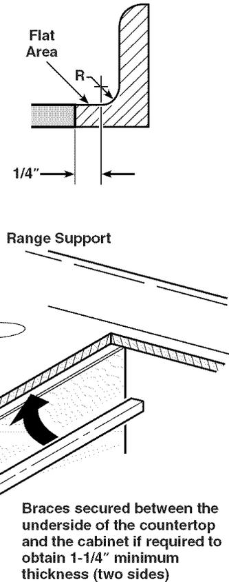
The Standard Installation of this Drop-In Range is to hang by the countertop on the side metal flanges under glass cooktop. **This Range must not be installed on a base or sub structure (2" x 4" support).**
