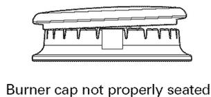
**C** Make sure the pins in the burner heads match the burner base indentations and that they are properly seated in them by rotating the heads until they are level.
