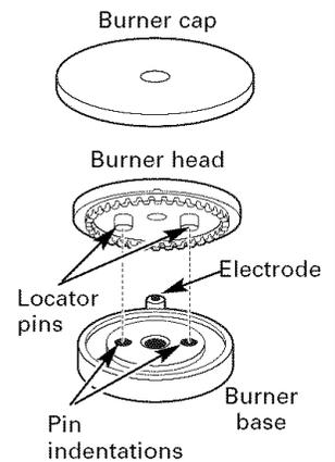
Make sure the slot in the burner head is positioned over the electrode. The burner cap has three to four pins. When replacing the cap, make sure none of the pins sits in the stability chamber.
