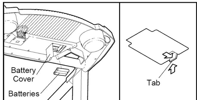
are touching the springs in the battery compartment. Close the battery cover, push up on the battery cover tab, and then push the tab forward as shown in the inset drawing. Make sure that the tab locks into place.
