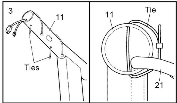
4. Place the Console Base (46) on the posts on the Upright. Make a loop with the indicated plastic ties and insert the two Wires (21) through the loops. Pull out only enough of the two Wires to connect them to the connectors in the Console Base. **Plug the Wires fully into the connectors.** Tighten the loops and cut off the excess plastic tie. **WARNING: Do not disconnect or connect the Wires while the treadmill power cord is plugged in.**
