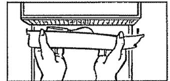
3. After replacing with same size bulb, reinstall panel and shelf
