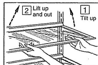
**To replace shelves,** select desired shelf height. With the shelf front raised slightly, engage the top lugs in the tracks at the rear of the cabinet. Then lower the front of the shelf until it locks into position.
