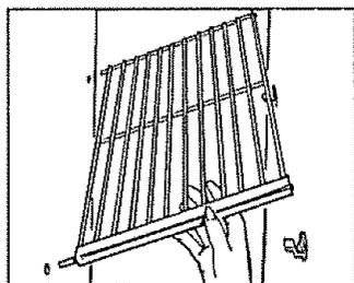
3. Select desired shelf height and insert rods into holes on left wall.
