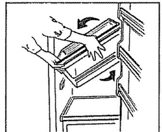
7. If tape holds bottom drawer cover to drawer supports, remove the tape. Pull drawer partway out. Reach in, push the rear of the glass up and, at the same time, back, until it clears front-corner retainers.
