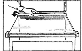
4. Pull the drawer partway out. Reach in, push the rear of the glass up; at the same time, push it back until it clears front-corner retainers.
