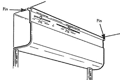
3. Pull the bottom of the light shield down and forward, then rotate the top up and off.
