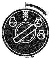
Engine "ON" Position (Normal Operating)
