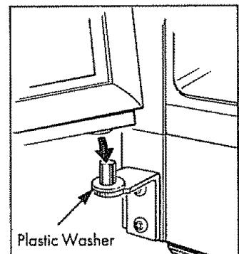
(b) Tilt the door towards the cabinet and gently push the door under the center hinge bracket and align with the hole in the center hinge bracket.
