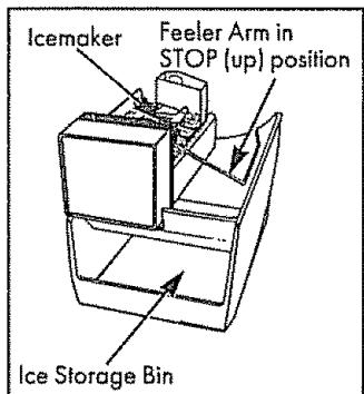
When the refrigerator has been connected to the water supply and the water has been turned on, position the freezer shelf for icemaking. Top lugs on the multi-position shelf should be in the 6th slot up from the bottom of the track; the 2-position shelf should be in the lower position. Then move the ice storage bin into place under the icemaker and move the feeler arm to the ON (down) position.
