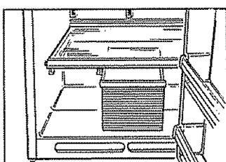
**3. Remove the glass cover.** Reach in, push the front of the glass cover up and, at the same time, pull it forward as far as it will come. Tilt it and take it out.
