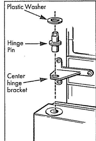
(c) Reinstall the hinge pin with a 3/8" socket and ratchet so it extends through the hole in the center hinge bracket and into the socket on top of the fresh food door.
