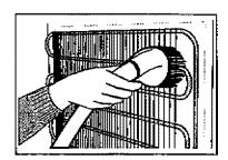
Clean the drain pan on the refrigerator compressor. Do not remove the drain pan!
