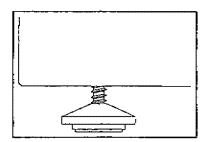
Two spacers attached to the appliance must be fitted onto the upper edge of the condenser, thus preventing the appliance from being installed too close to the wall. Spacers are manufactured for all-purpose function depending on the distance of the condenser from the wall. Therefore turn spacers correspondingly and fix them to the appliance.
