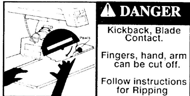
Fig. 101 - Kickback, Blade Contact Safety Sign
