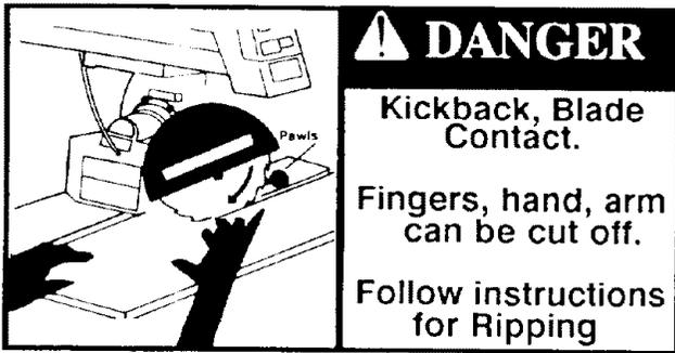
Fig. 109 - Kickback, Blade Contact Safety Sign
