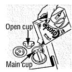
Be sure the Dial is **OFF** before adding detergent. Otherwise, the detergent cup will not close and latch properly. Add detergent then close the main cup.
