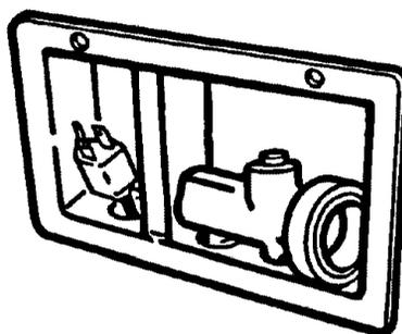
3. Pull down on the locking collar while lifting the hose connector onto the faucet adapter.
