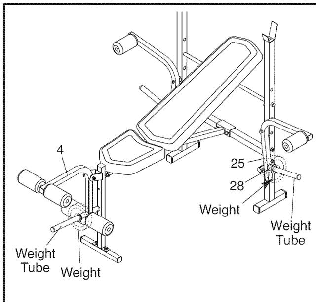
**▲ WARNING:** When using the Leg Lever (4), place a barbell with the same amount of weight on the weight rests to balance the bench.
