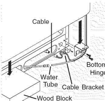
**NOTE:** If refrigerator has been used, have a container ready to catch excess water from tube.
