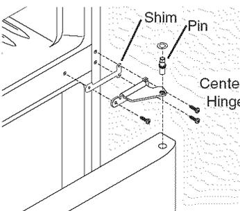
5. Remove the bottom hinge screws and hinge, holding the door as its weight rests on the wood block. Lay the door on its side to avoid damage to cable and tube.
