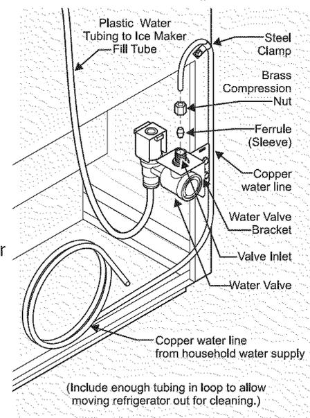
**IMPORTANT:** It takes approximately 24 hours for the ice maker to begin producing ice. Air in new plumbing lines may cause ice maker to cycle two or three times before making a full tray of ice. New plumbing may cause ice to be discolored or have poor flavor. Discard ice made during the first 24 hours. After connecting the water supply, refer to "How to Prime the Water Supply System" for important information about priming an empty water supply system.
