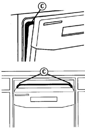
Open door about 3 inches (7.6cm) and check for equal spacing (C) between inner door and tub sides. If spacing is not equal, loosen bracket screws and shift tub. Tighten bracket screws. Remove newspaper or towel from dishwasher.
