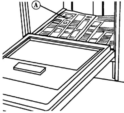
Open dishwasher door and remove all shipping materials. Remove bottom rack. Place newspaper (A) or towel over bottom of dishwasher to prevent screws from falling into pump area when securing dishwasher to countertop.
