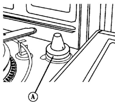
Read the Use and Care Guide that came with your dishwasher. Reconnect power supply to dishwasher. Set the dishwasher to run the "Normal" cycle. Start dishwasher and allow it to run for 2 minutes. Open dishwasher door. The water level should be deep enough to cause the float (A) to float on the water. If the water level is correct, close the door and allow the dishwasher to complete the cycle. If the dishwasher does not fill to the proper level, check the following:
