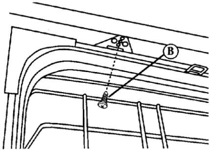
The dishwasher **MUST** be secured to countertop or floor to keep it from tipping when door is opened.
