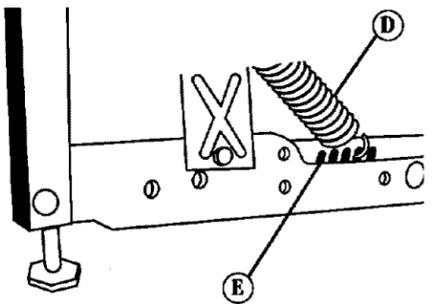
Open and close door several times. The door should open and close easily. If door closes too quickly or falls open, adjust door springs (D) by moving spring ends to different holes (E) in base.
