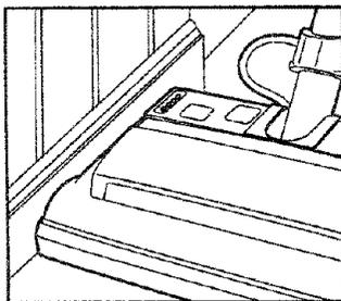
Active brush edge cleaners are on both sides of the POWER-MATE™. Guide either side of the POWER-MATE™ along baseboards or next to furniture to help remove dirt trapped at carpet edges.
