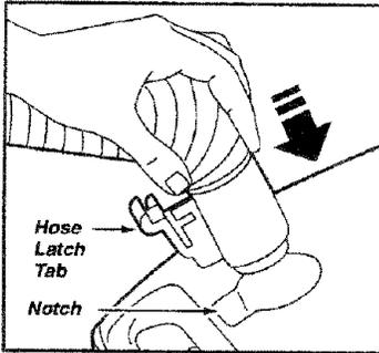
1. Line up the hose latch tab and notch in canister hood and insert hose into canister until it snaps in place.
