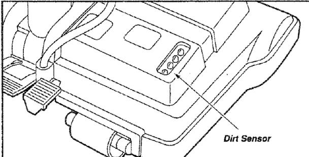
The lights give you an indication of the amount of dirt particles that are passing thru the sensor on its way to the dust bag.
