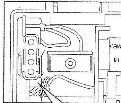
5. **NOTE:** Be sure that the board is upright and the wires are tucked back as shown.
