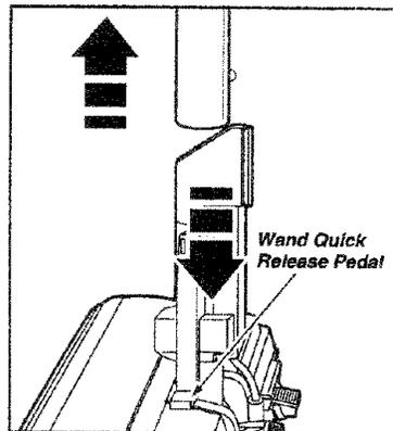
2. Press wand release pedal with foot and pull the wands straight up out of POWER-MATE™.
