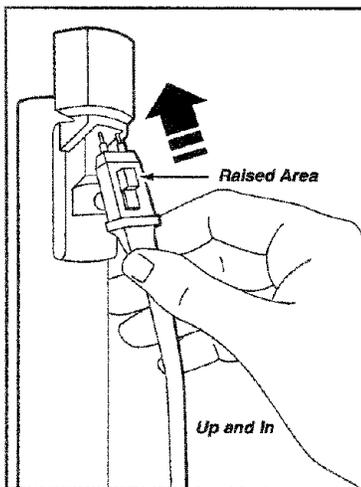
2. Connect POWER-MATE™ plug and cord as shown. **DO NOT force.** Raised area of plug must be toward hand.
