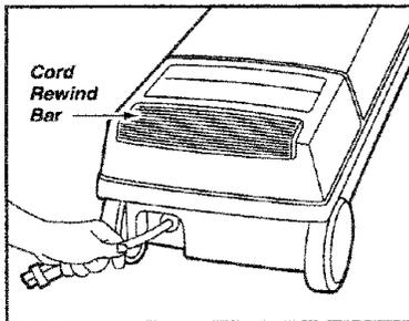
1. Pull cord out of canister to desired length. The cord will not rewind until the cord rewind bar is pushed.
