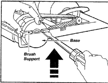
5. Carefully insert and twist screwdriver at each brush support to free brush from base.
