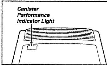
The light comes on whenever the airflow becomes blocked, dust bag needs changing or canister safety filter needs cleaning.
