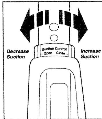
The suction control allows you to change the vacuum suction for different fabric and carpet weights. Opening the control decreases suction for draperies and lightweight rugs, while closing the control increases suction for upholsteries and carpets.
