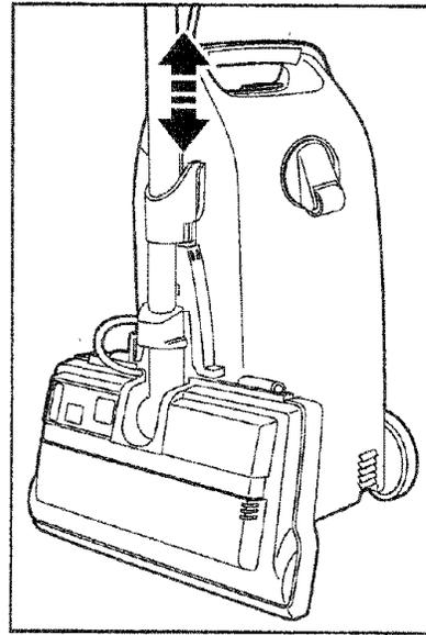
The lower wand has a "U" shaped flange in the area where the power cord attaches. The base has a "U" shaped slot near the front caster.
