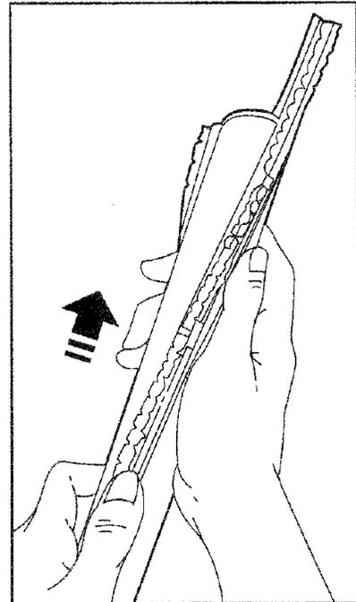
5. Reassemble brush assembly. To line up screw holes in dowel, sprocket and end brush, be sure beater bar portion of end brush lines up with beater bar on brush dowel.
