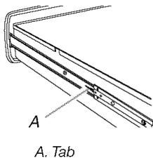
3. Press the tab down on the right side of the drawer and lift tab up on the left side of the drawer at the same time. Then pull drawer out another inch to disengage latch.
