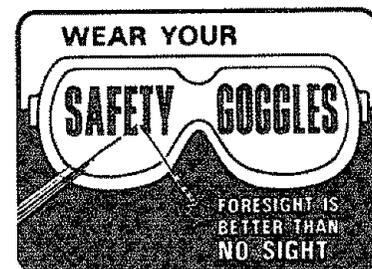
Any power sander can throw foreign objects into the eyes. This can cause permanent eye damage. Wear safety goggles (not glasses) that comply with ANSI Z87.1 (shown on package). Everyday eyeglasses have only impact resistant lenses. They are not safety glasses. Safety goggles are available at Sears retail catalog stores. Glasses or goggles not in compliance with ANSI Z87.1 could seriously hurt you when they break.
