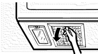
To remove, slide it to the rear using the tab. Pull it down and out.
