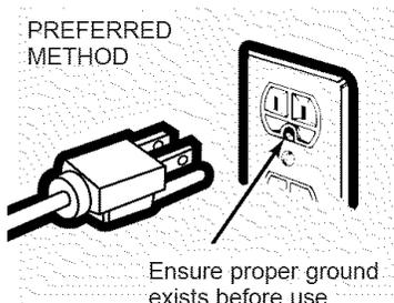
**⚠ WARNING—Improper use of the grounding plug can result in a risk of electric shock.**
