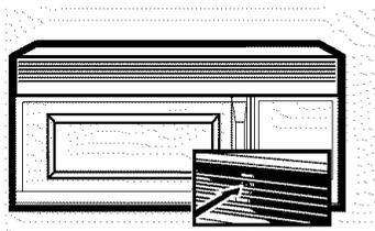
Remove the top grille by taking out the 2 screws that hold it in place.
