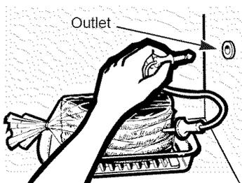
**1 Insert the probe in the roast and attach it securely into the oven wall outlet.**
