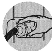
Hand tighten couplings – hot to hot, cold to cold.
