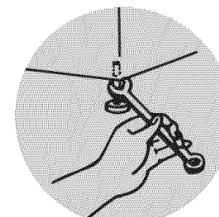
If level, use a 3/8" (14 mm) open-end wrench to turn the nuts on the feet tightly against the washer cabinet.
