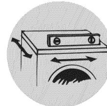
Check the levelness of the washer, side to side and front to back.
