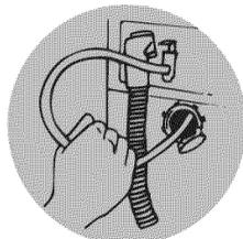
Pull the power cord through the opening and close the hole with the attached cap.
