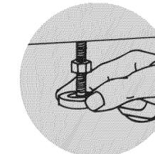
Push on the upper front panel to be sure that the washer is on the rear feet. Lower right front foot to floor. By hand, firmly rotate foot up to an additional 1/2 turns.
