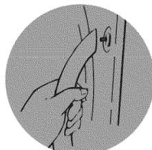
Insert the 2 screws through the holes in the door. Place the plastic washers onto the screws. Attach the handle by hand tightening the screws, first the top then the bottom. Push the handle against the door. Using a Phillips screwdriver, tighten the screws.
