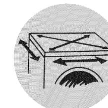
Rock washer gently front to back, side to side and diagonally to make sure that all four feet are in firm contact with the floor.
