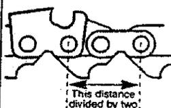
Pitch refers to chain measurement. A chain's pitch is the distance between any three of its rivets divided by two.
