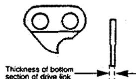
Gauge refers to thickness of that portion of drive link which fits into saw bar groove.
