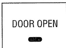
If the signal light on the DOOR ALARM pad is glowing, the beeper alarm is set. If it's not, touch the pad to turn it on.
