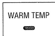
From then on, the red light will glow whenever temperatures inside get too high for proper food storage. If this happens, open the doors only when absolutely necessary, and close them as quickly as possible.
