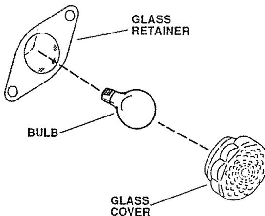
**Be sure that the light switch is in the off position. Do not touch hot oven bulb. Do not touch oven bulb with wet hands. Do not wipe oven light area with wet cloth.**
