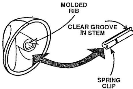
All control knobs may be removed for easy cleaning by pulling the knob straight off the stem. Be sure that the knob is in the OFF position before removal.
