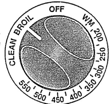
2. When broiling is finished, turn the OVEN CONTROL KNOB to the "OFF" position.
