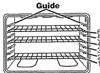
**Always place oven racks in the proper position while oven is cool.**
