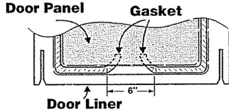
It is normal for your oven door to give the appearance of not having a good seal against the oven. This is due to the gasket. The location of the gasket on the oven door maintains a good seal and prevents any heat loss.
