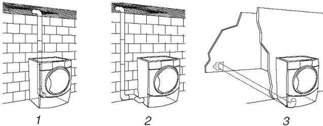
1. Standard rear offset exhaust installation
