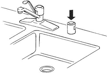
The drain air gap is usually located on top of the sink or countertop near the dishwasher. To order a drain air gap, contact your local dealer; or call the Customer Interaction Center and ask for Part Number 300096.
