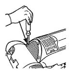
6. Snap lens cover back into place and secure the headlight lens by replacing the two screws.
