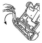
Rotate/pivot the nozzle guard and pull off
