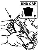
With new belt in place, pull and slide brushroll into nozzle making sure that the brushroll end caps are in the correct orientation (see diagram for end cap orientation). Rotate brushroll manually to make sure belt is properly aligned.
