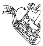
Secure by aligning the three (3) tabs in the base slots. To reattach nozzle guard, rotate/pivot back into position.
