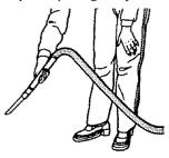
If additional length is needed, use the telescoping wand and crevice tool. Use telescoping wand and crevice tool together or separately.
