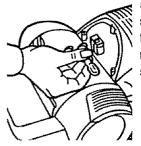
5. Pull bulb out of socket. Do NOT twist. Gently push replacement bulb into socket to replace.
