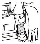
**3.** Disconnect the hose by pulling down on the lower intake hose cuff.
