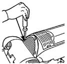
3. Remove the two (2) screws from the lens cover.
