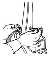
2. Push handle plug onto the front of cleaner. Insert the one (1) screw into the back of the handle and tighten, making sure the handle plug is secure.
