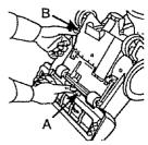
To secure nozzle guard, push lock B down to lock position. Slide lock A into lock position, to the right.
