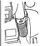
2. Rotate lower intake hose cuff clockwise into the unlock position.
