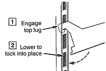
**To relocate shelves:** Select desired shelf height. With shelf front raised slightly, engage top lugs in tracks at rear of cabinet. Then lower front of shelf until it locks into position.
