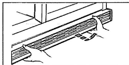
**To adjust rollers, remove the base grille by grasping it at the bottom and pulling it out.**
