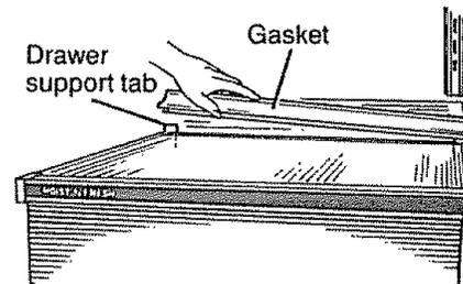
2. Remove the flexible gasket at the rear of the Moist 'n Fresh drawer. Lift each end straight up until the slots on the gasket are free of the drawer support tabs.
