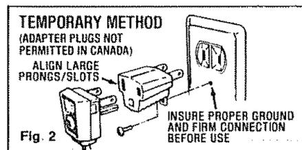
The larger slot in the adapter must be aligned with the larger slot in the wall outlet to provide proper polarity in the connection of the power cord.
