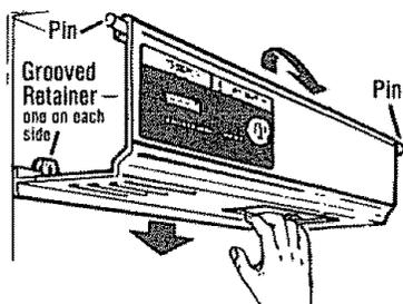
3. Pull bottom of light panel down about 1/4"—just enough to disengage lip at rear from grooves in retainers on rear wall.
