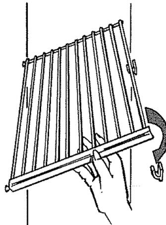
**If shelf supports at desired level on right wall do not have tabs,** merely lower shelf into place on supports.
