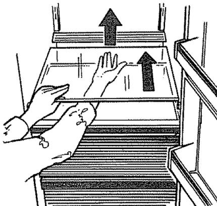
3. Pull the drawer part-way out. Reach in, push the rear of the glass up and, at the same time, push it back until it clears the front corner retainers.
