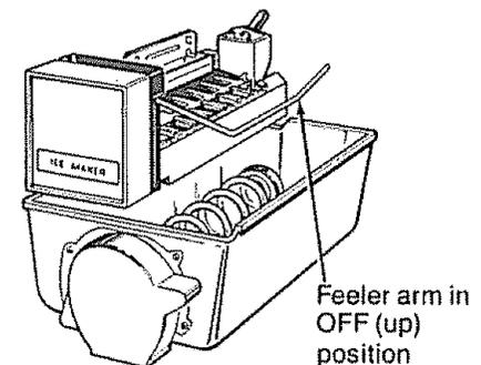
When water supply has been connected to icemaker, move feeler arm to ON (down) position.
