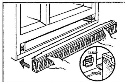
**To replace base grille, align prongs on back of grille with clamps in cabinet and push forward until grille snaps into place.**
