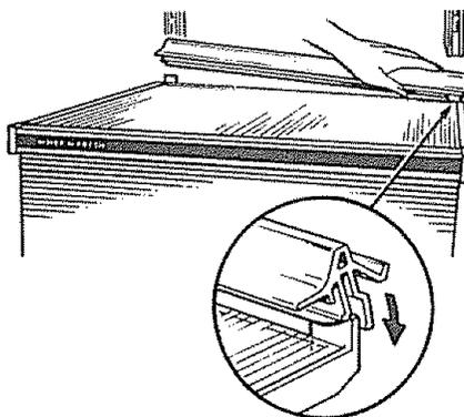
9. Reinstall the gasket at the rear of the Moist 'n Fresh drawer. Fit the end of the plastic drawer support into the slot on the gasket, with the rubber gasket flap facing you. Make sure the gasket snaps into place.
