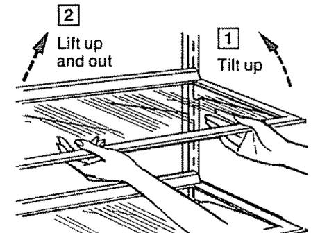
**To remove shelves:** Tilt shelf up at front, then lift it up and out of tracks on rear wall of refrigerator.
