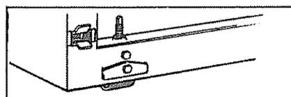
When adjusting front rollers for proper door closure, we recommend that the bottom front edge of the cabinet be approximately 5/8" from the floor.
