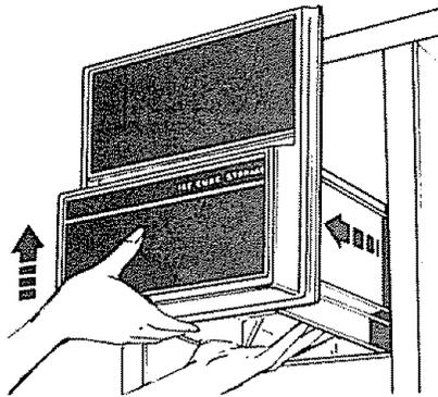
Lift the left corner to free the bin from the shelf, and pull the bin straight out while supporting it at front and back.
