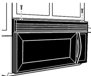
2. Tilt vent grille forward and lift to remove.
