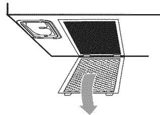
2. Replace grease filters by inserting the end without the tab into the frame. Swing other end up and slide into position.
