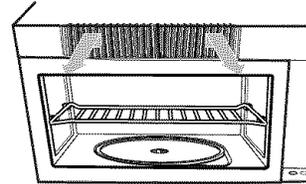
4. Replace the charcoal odor filter by positioning the new filter in the slot. “This side out” printed on the edge of the filter should be facing out. Then replace the vent grille by aligning the bottom tabs and snapping it back into place.
