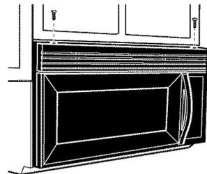
3. Tilt vent grille forward and lift to remove.
