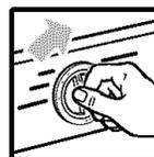
**NOTE:** If the door is latched, you will hear the cycles start and stop as the Cycle Control knob passes each cycle mark. This is normal and does not hurt the dishwasher. If you prefer, you can set the Cycle Control knob with the door unlatched.
