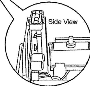
6. Rotate cover back. Press cover firmly until side and rear tabs snap into place. Turn Power-Mate® upside down and replace two (2) cover screws.
