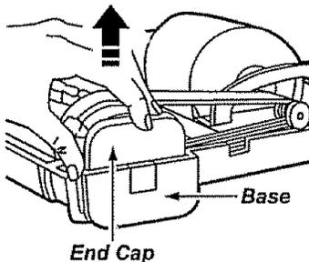
6. Lift agitator assembly out and remove worn belt.
