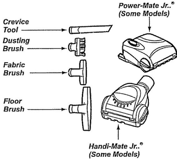
**NOTE:** All models have one set of attachments in the canister. Some models have an additional set, which can be kept in the accessory bag for garage use or other dirty areas.
