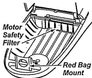
6. Check and replace, if necessary, the motor safety filter.
