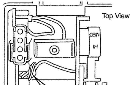
5. **NOTE:** On dirt sensor models be sure that the board is upright and the wires are tucked back as shown.
