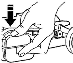
2. Place agitator assembly back into Power-Mate®.
