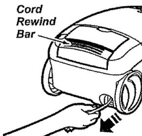
1. Pull cord out of canister to desired length. The cord will not rewind until the cord rewind bar is pushed.
