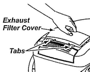
4. Replace the exhaust filter cover by engaging the two tabs on the rear and pushing down in front until it snaps closed.
