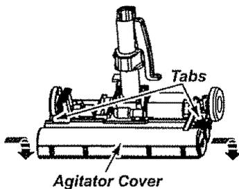
4. Line up front of cover and base. Rest cover on front edge of base as shown.
