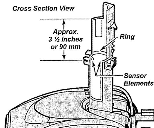
2. As indicated by the illustration, the two dirt sensor elements are located on the inside of the swivel, approximately 3 1/2 inches/90 mm down, (note the arrows). Each element should be cleaned periodically. To reach the sensor elements, use a small brush such as a bottle brush. Brush each sensor element several times to remove dust and dirt.
