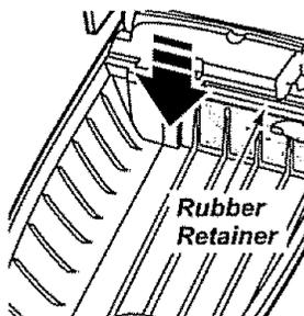
2. Replace the filter, **rough side out**, facing the dust bag, by sliding it back into place under the ribs in the bag cavity. Tuck filter in so that it fits completely under the rubber
