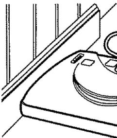
Active brush edge cleaners are on both sides of the Power-Mate®. Guide either side of the Power-Mate® along baseboards or next to furniture to help remove dirt trapped at carpet edges.
