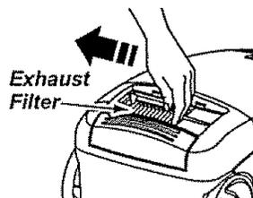
2. Slightly push the exhaust filter cartridge to the side, as shown in the illustration, and pull up to remove.
