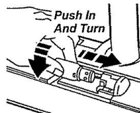
3. Push in and turn bulb clockwise, to replace. Bulb must not be higher than 15 Watts(130 Volts).
