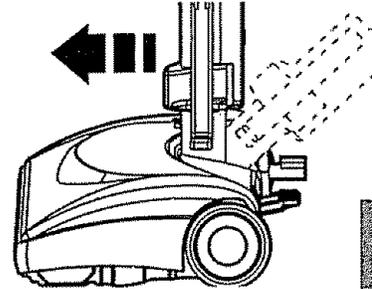
2. Press wand quick release pedal with foot and pull the wands straight up out of Power-Mate®.
