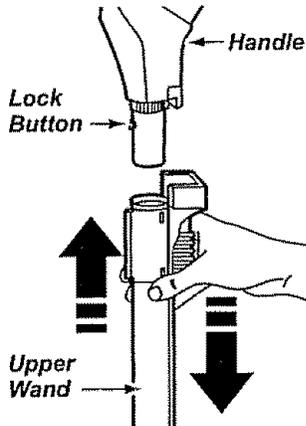
**NOTE:** If the Power-Mate® is attached, turn cleaner off before removing handle from wands.
