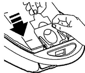
Tuck the bag securely into the bag cavity so that none of it is able to be pinched by the hood.
