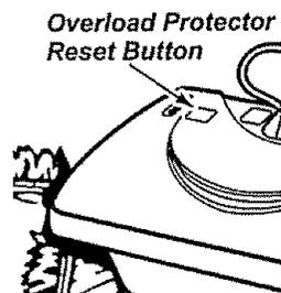
**To correct problem:** Turn off vacuum, remove obstruction, then press reset button.
