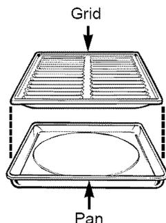
**If food has burned on**, sprinkle the grid with detergent while hot and cover with wet paper towels or a dishcloth. Soaking the pan will remove burned-on foods. The broiler pan and grid may be cleaned with a commercial oven cleaner.
