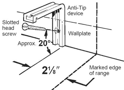
2. Locate the outside edge of the device  $2\frac{1}{8}$ " toward the center of the range from the marked edge of the range.
