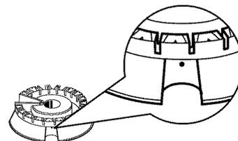
The slits in the burner heads of your range must be kept clean at all times for an even, unhampered flame.
