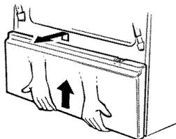
**To replace**, insert the two slots at the bottom of the panel onto the two tabs at the base of the range and push the top of the panel forward to engage the spring clips.
