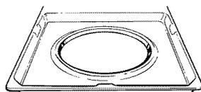
When replacing the drip pans, make sure they are in the correct position.
