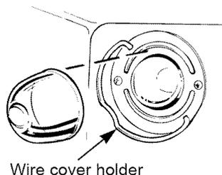
DO NOT REMOVE ANY SCREWS TO REMOVE COVER.
