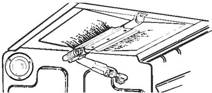
The flames for the top (broil) burner should be steady with approximately 1" blue cones and should not extend out over the edges of the burner baffle.
