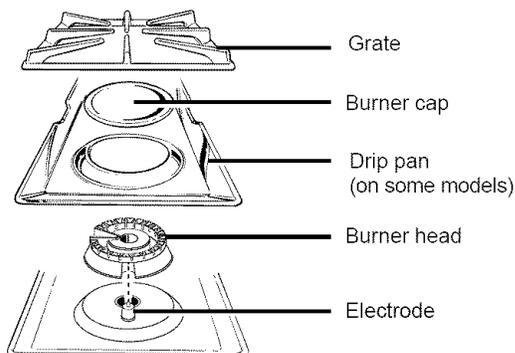
Turn all controls OFF before removing the burner parts and drip pans (if so equipped).
