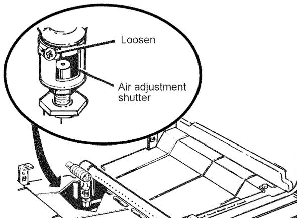
The shutter for the bottom (oven) burner is near the back wall behind the kick panel. Remove the panel. See the Care and Cleaning section in this guide.
