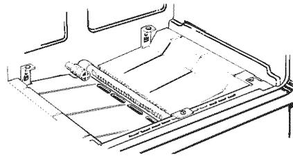
To determine if the bottom burner flames are burning properly, remove the oven bottom. Flames should have approximately 1" blue cones and, if range is supplied with natural gas, should burn with no yellow tipping. (With most LP gas, small yellow tips at the end of outer cones are normal.) Flames should not lift off burner ports. If lifting is observed, gradually reduce air shutter opening until flames are stabilized.
