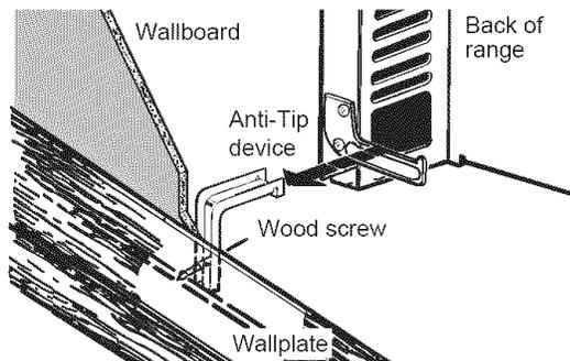
5. Slide the range against the wall, and check for proper installation by grasping the front edge of the cooktop and carefully attempting to tilt the range forward.
