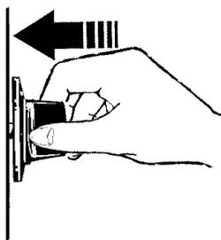
When one burner is turned to LITE, *all* the burners spark. Do not attempt to disassemble or clean around any burner while another burner is on. An electric shock may result, which could cause you to knock over hot cookware.
