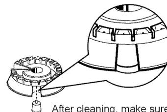
Replace the burner heads and caps. Make sure that the heads and caps are replaced in the correct location. There is one small, 2 medium and one large head and cap.
