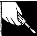
**ADJUST BROIL AND OVEN BURNER AIR ADJUSTMENT SHUTTERS ON MODELS WITH A STORAGE DRAWER, IF NECESSARY (See Step 9 if your range is equipped with a broiler drawer.)**
