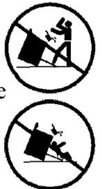
To check if the device is installed and engaged properly, carefully tip the range forward. The Anti-Tip device should engage and prevent the range from tipping over.
