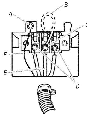
A. External ground conductor screw
