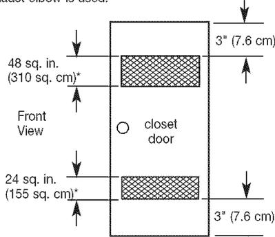
\*Opening is the minimum for a closet door. Louvered doors with equivalent air openings are acceptable.
