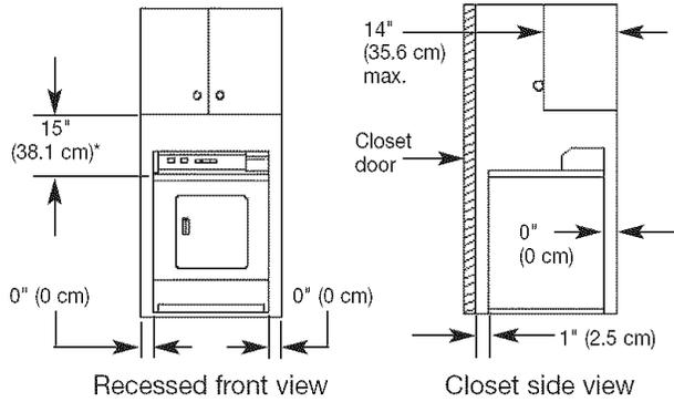
Additional clearances for wall, door and floor moldings may be required or if external exhaust elbow is used.
