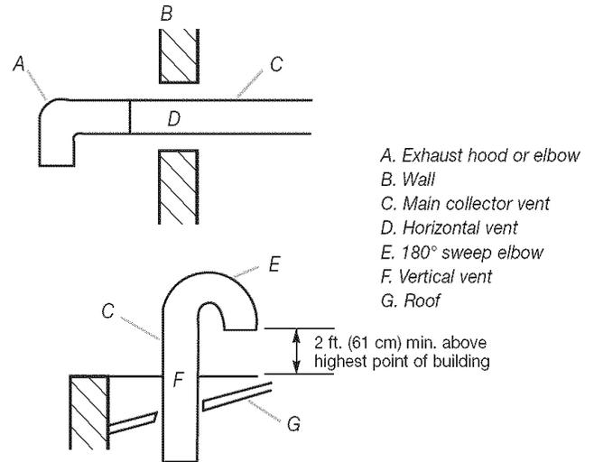
Do not install screening or cap over the end of the vent.
