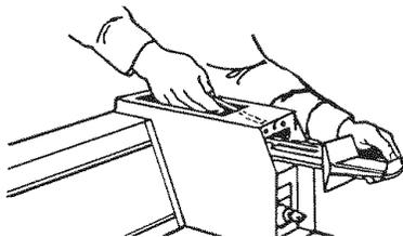
For dryers using coin slides, use adapter kit supplied with dryer.
