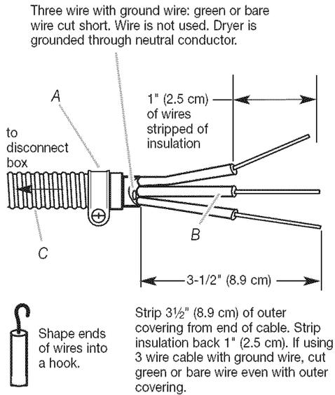
Three wire with ground wire: green or bare wire cut short. Wire is not used. Dryer is grounded through neutral conductor.
