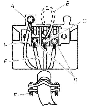
A. External ground conductor screw
