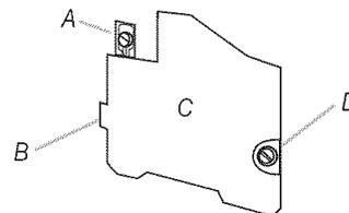
A. External ground conductor screw
