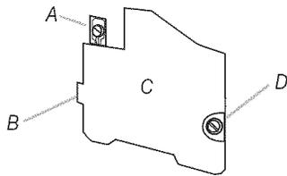
A. External ground conductor screw
