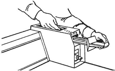
For dryers using coin slides, use adapter kit supplied with dryer.
