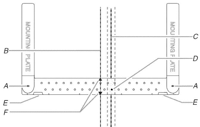
**NOTE:** If wall stud is within 6" (15.2 cm) of the vertical centerline (see “Mark Rear Wall” section), only recirculation or roof venting installation can be done.
