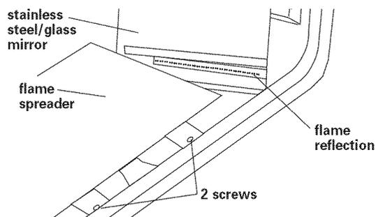
You can check the burner flame by removing the flame spreader or by using a mirror.
