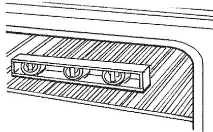
**8.** Place rack in oven. Place level on rack, first side to side; then front to back. If range is not level, pull range forward until rear leveling leg is removed from the anti-tip bracket. Use 3/8" drive ratchet and channel lock pliers to adjust leveling legs up or down until range is level. Push range back into position. Check that rear leveling leg is engaged in anti-tip bracket.
