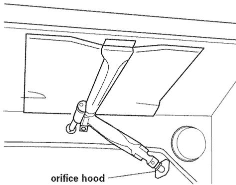
**5. Broil burner:** Use 1/2" combination wrench to turn the orifice hood down snug onto pin (approximately 2 to 2-1/2 turns). **DO NOT OVERTIGHTEN.** The burner flame cannot be properly adjusted if this conversion is not made.
