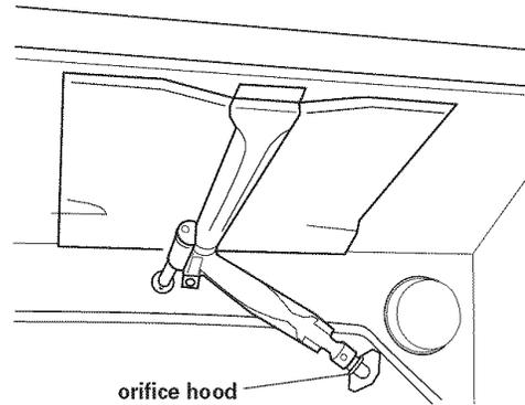
**5. Broil burner:** Use 1/2" combination wrench to loosen orifice hood away from pin (approximately 2 to 2-1/2 turns). The burner flame cannot be properly adjusted if this conversion is not made.
