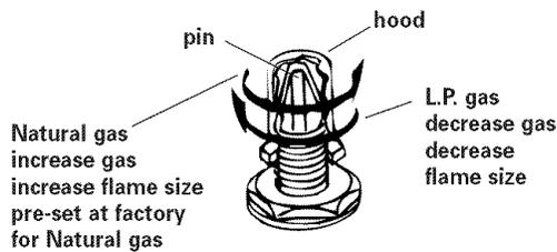
**4. Oven burner:** Use 1/2" combination wrench to loosen the orifice hood away from pin (approximately 2 to 2-1/2 turns). The burner flame cannot be properly adjusted if this conversion is not made.
