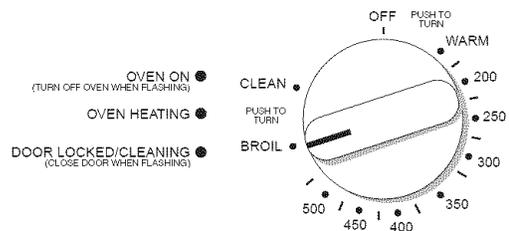
Push in and turn the oven selector control knob to "BROIL." If the burner fails to light due to air remaining in the gas line, reset the oven control by turning selector knob to "OFF" and then again to "BROIL".
