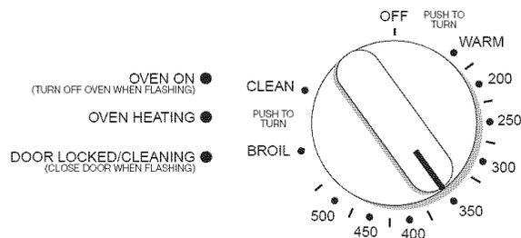
Push in and turn the oven selector control knob to "350". If the burner fails to light due to air remaining in the gas line, reset the oven control by turning selector knob to "OFF" and then again to "350".
