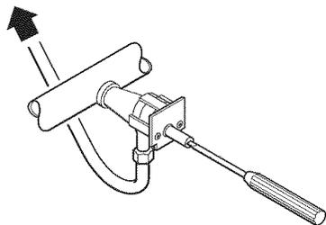
**16.** Push in and turn each cooktop control knob from "LIGHT" to "LOW" setting quickly. The low flame should be a minimum, steady blue flame. If flame needs to be adjusted, turn control knob to the "LOW" setting and remove control knob. Insert a small flat-blade screwdriver into the valve stem. Turn the valve screw to obtain the smallest flame that will not go out when the control of a cold burner is quickly turned from "HIGH" to "LOW". Repeat for other cooktop burners as needed.
