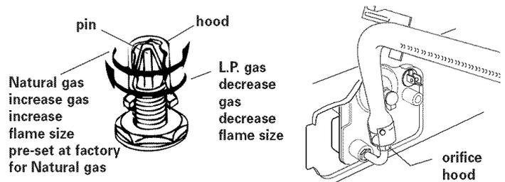
**4. Oven burner:** Use 1/2" combination wrench to turn the orifice hood down snug onto pin (approximately 2 to 2-1/2 turns). **DO NOT OVERTIGHTEN.** The burner flame cannot be properly adjusted if this conversion is not made.
