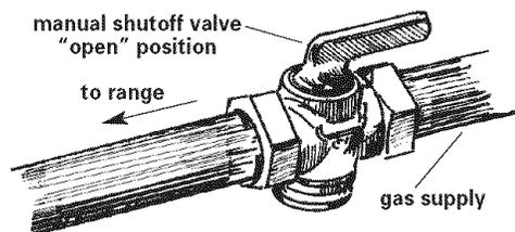
**Shutoff valve:** The supply line must be equipped with a manual shutoff valve. This valve should be located in the same room as the range and should be in a location that allows ease of opening and closing. The valve is for turning on or shutting off gas to the range. **Do Not block access to shutoff valve.**
