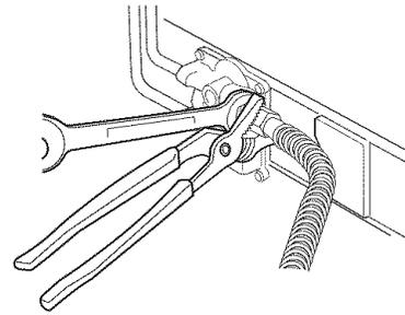
**10.** Use 15/16" combination wrench and channel lock pliers to attach the flexible connector to the adapters. Check that connector is not kinked.
