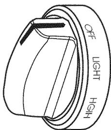
**15.** Push in and turn each surface unit control knob to "LIGHT" position. The flame should light within 4 seconds. Turn control knob to "HIGH" position after burner lights.
