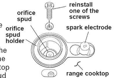
Note: Reinstall one of the screws through the range cooktop to hold orifice spud holder in place while removing and replacing orifice spuds.
