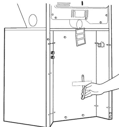
2. Tilt the washer/dryer forward. Move each of the 2 rear legs in an up-down motion to check the self-adjusting leveling legs for free movement. This is required for proper leveling. Gently lower the washer/dryer to the floor.
