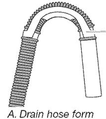
2. Put hooked end of drain hose into laundry tub or standpipe. Rotate hook to eliminate kinks.
