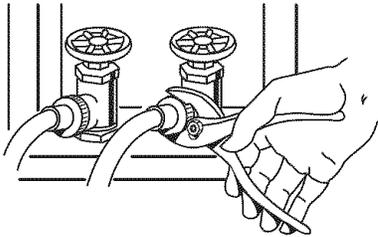
**NOTE:** Do not overtighten or use tape or sealants on valve. Damage to the valves can result.
