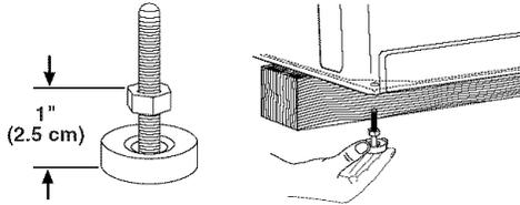
3. Screw the feet into the correct holes at the front corner of the washer/dryer until the nuts touch the washer.
