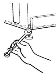
3. Tilt the washer/dryer forward until the rear of the washer/dryer is at least 4" (10.2 cm) off the floor. You may hear the self-adjusting rear feet click into place. Lower the washer/dryer to the floor. Check the levelness of the washer/dryer with a level as shown above.
