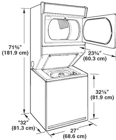
\*Most installations require a minimum 5" (12.7 cm) clearance behind the dryer for the exhaust vent with elbow. See "Venting Requirements."
