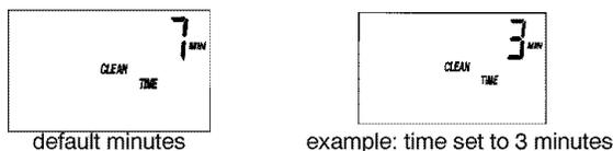
■ **CLEAN feature minutes:** If you are using this feature, the length of the extra backwash cycle automatically sets to 7 minutes. However, you can ad-
