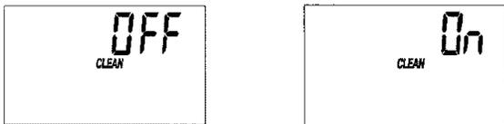
■ **CLEAN:** This feature is beneficial on water supplies containing iron and/or high amounts of sediments (sand, silt, dirt, etc.). When set to ON, a backwash and fast rinse cycle will occur first, preceding the normal regeneration sequence (see page 2-4). This provides extra cleaning of the resin bed before it is regenerated with the salt brine. To conserve water, if your water supply does not contain iron or sediments, be sure this feature is set to OFF.
