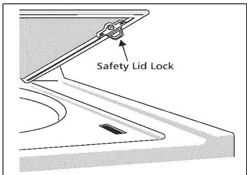
**⚠ WARNING** To avoid serious personal injury, do not operate washer if safety lid lock is missing or damaged.
