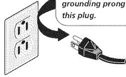
Power supply cord with 3-prong grounding plug
