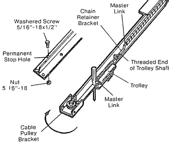
As a permanent trolley stop, insert 5/16" washered screw into remaining hole in Tee rail front. Tighten securely with 5/16" nut. **REMOVE TEMPORARY STOP INSERTED IN STEP 2.**
