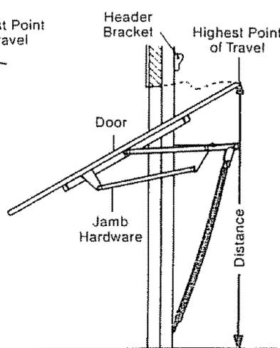
Locate height for header bracket by opening door to highest point of travel as shown. Measure distance from top of door to floor. Subtract actual height of door. Add 8" to the remainder. See example below.
