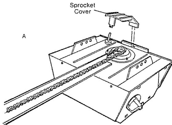
**PROCEDURE:** Attach sprocket cover to chassis as shown in Illustrations (A) and (B). Insert back tab in chassis slot. Then bend cover forward and insert front tab in slot provided on mounting plate.
