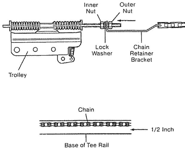
**PROCEDURE:** Thread inner nut along shaft toward trolley. Tighten chain and cable by turning outer nut in the same direction as shown.
