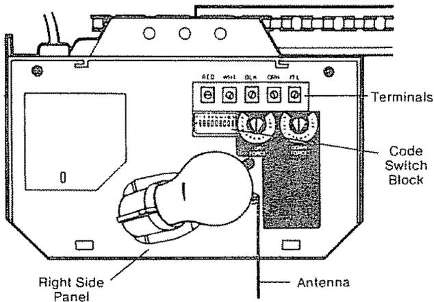
**RADIO CONTROLS** consist of two 3-channel transmitters and a receiver. The coded signal is factory preset.
