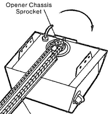
Install Chain and Cable in This Direction
